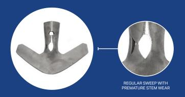
"We are pleased with the performance of our Blue Armour Sweeps. We were hoping for 30% more usable life than the competitor's sweep but we are getting closer to 50%. The wear pattern is better because Blue Armour retains the leading tip of the sweep much longer. This keeps us at a more consistent depth."
