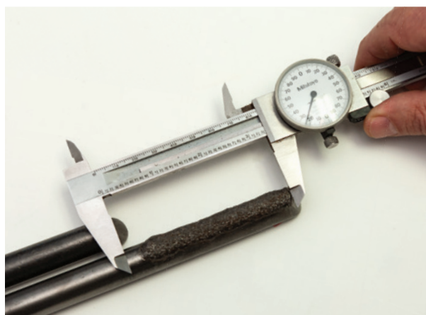
10,000 acres of wear comparing a MAX LIFE tine to a regular tine.
