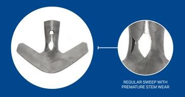
"It was a tough spring for wear on sweeps but the BTT sweeps are a good product. I think they wore more evenly and slightly longer than the John Deere sweep, hard to tell how much longer they lasted due to the dry soil. I liked the longer neck on them as well. The bottom bolt gets wear on it before they need to be changed but the longer neck seems to minimize that."
