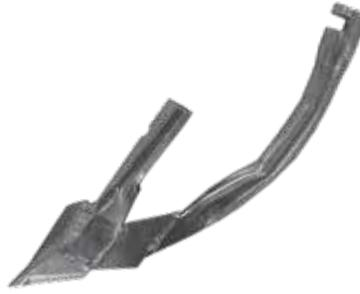
**200-KNF-7542****SINGLE SHOOT OPENER****FITS:** 200 Series Speed-Loc™**FERTILIZER TYPE:** Granular**TUBE SIZE:** 1-1/4" (32 mm) O.D.**TIP OPTIONS:** The high-chrome welded tip is long lasting and provides excellent penetration.**INSTALLATION DRIVER:** 100-DRV-1010
